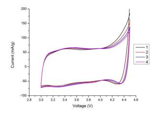
Figure 1. Current vs. Voltage curve at a scan rate of 1.0 mV/s.
