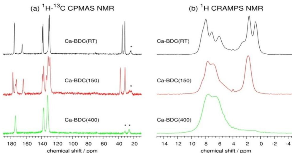
Figure 1.  $^1\text{H}$ - $^{13}\text{C}$  CPMAS (a) and  $^1\text{H}$  CRAMPS (b) NMR spectra of as-prepared and thermally treated Ca-BDC material. The spectra indicate that the framework is rearranged during heating, that the environment of DMF molecules is changed upon heating to 150 °C, and that DMF is entirely removed upon heating to 400 °C. Additional information about the detachment of DMF from Ca centres was obtained by  $^1\text{H}$ - $^1\text{H}$  2D NMR correlation experiment.
