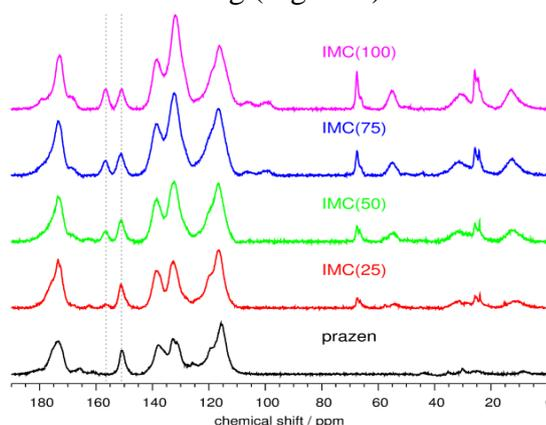
Figure 3.  $^1\text{H}$ - $^{13}\text{C}$  CPMAS NMR spectra of Al-MIL-101/IMC drug-delivery systems. The systems contain different amounts of drug (IMC). The dotted lines denote two well-resolved signals of IMC (the left signal) and
