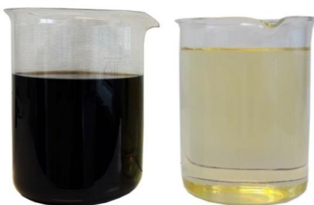
Figure 1. Comparison of the raw leachate sample (left) and after treatment with lime and aeration (right) [3-5].
